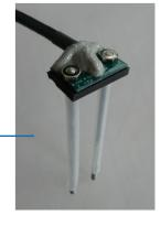
Point Moisture Measurement Sensor (PMM) is used for moisture content measurement of timber.
