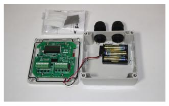
Data loggers that communicate wired or wirelessly to a gateway device in the building.
