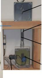
String Pot is a sensor for vertical, horizotal and/or diagonal displacement monitoring
