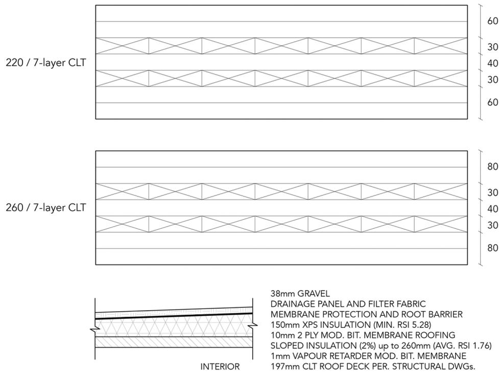
Fig. 5. Typical CLT roof panels (above) and assembly (below) – adapted from TRCA [8].
