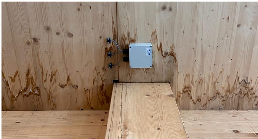
Fig. 7. Instrumentation installation at underside of CLT roof deck at panel edges
