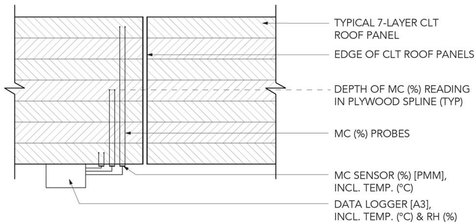
Fig. 6. Typical moisture content measurement instrumentation diagram.
