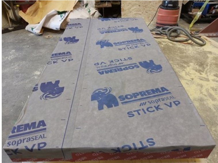
Figure 15. CLT panel covered with a self-adhesive, vapour-permeable membrane, with four edges sealed with an impermeable membrane.
