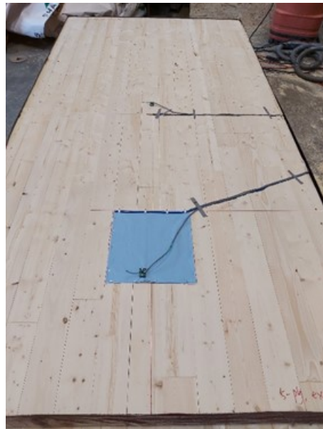
Figure 3. A paper-based external wetting pad together with a plastic tube and sensors installed on the exterior surface of a CLT panel.
