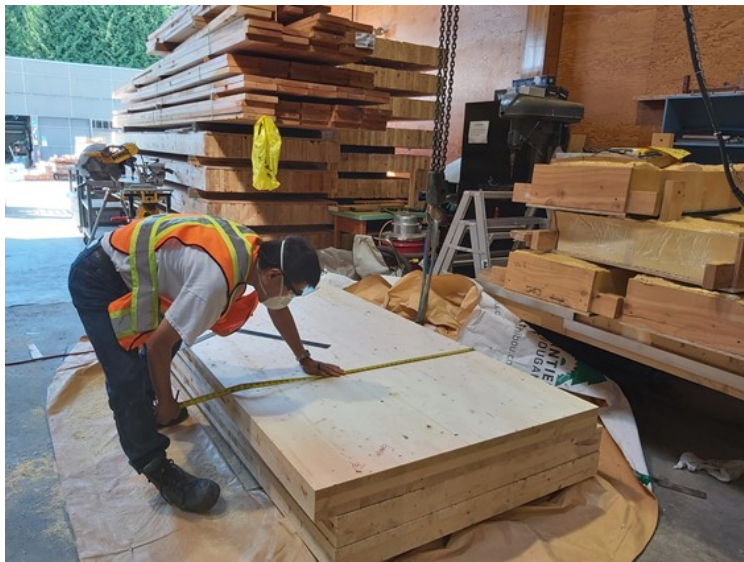
Figure 14. CLT panel being pre-prepared for instrumentation and assembly.
